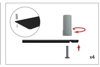
**Step 4:** Push banner stand frame onto posts of flat base or optional feet. Press evenly on both sides to make easier for the frame to go on.
