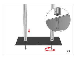
**Step 2:** Tighten the screws on the connector bars to secure the 3-piece support pole together.
