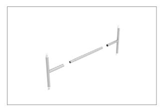
**Step 14: Turn. Position. Lock.** Insert tensioning pole into the bottom of display. Keep the pole flat until the entire pole fits inside the frame. **Turn** the pole 45°.
