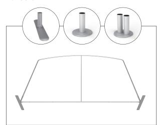
**Step 5:** Unzip print and lay image face up. Slide print onto frame like a pillow case. Pull and stretch the graphic below the bottom cross bar and zip closed under the cross bar.
