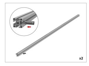
**Step 5:** To install the VESA Mount insert the screw through the hole and into the wedge. Place the wedge into the groove of the pole and rotate. Tighten screw.
